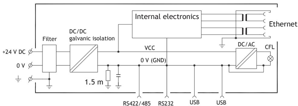
The operator panel has galvanic isolation against the 24 V DC feed but no galvanic isolation between the communication ports for RS232, RS422/485 and USB. Only the Ethernet connection has galvanic isolation.
