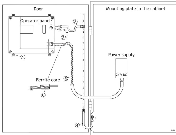
The mounting clamps of the operator panel do not provide a secure grounding connection between the panel and the device cabinet, see 1 in drawing above.
