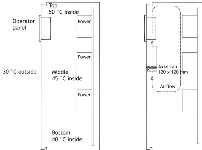
In most cases, the ambient temperature for the operator panel is significantly higher than the device cabinet's ambient temperature.
