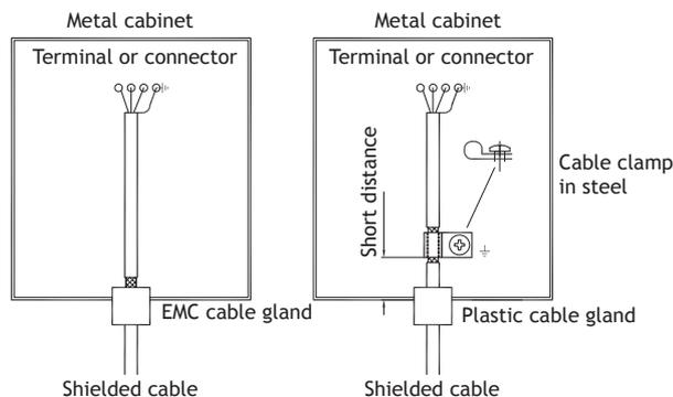
1. Use an EMC cable gland or regular plastic cable gland, remove the outer jacket and connect the shield to the installation plate with a 360° metal cable clamp.
