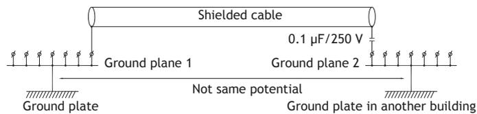
With longer distances, there is a risk that the ground potential may be different. In that case, the shield should only be connected at one end. A good alternative is to connect the other end of the shield to the ground via a 0.1  $\mu\text{F}/250\text{ V}$  plastic capacitor. Both ends are then connected to the ground in terms of HF, but only connected to the ground at one end in terms of LF, thus avoiding the 50/60 Hz grounding loops.
